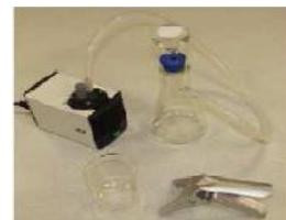
Gambar 2.2 Pompa vakum manual
